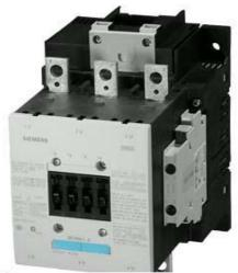
CONTACTOR, 75KW/400V/AC-3, AC(40...60HZ)/DC OPERATION UC 110...127V AUXIL. CONTACTS 2NO+2NC 3-POLE, SIZE S6 BAR CONNECTIONS CONVENTIONAL OPERATING MECHAN. SCREW TERMINAL
